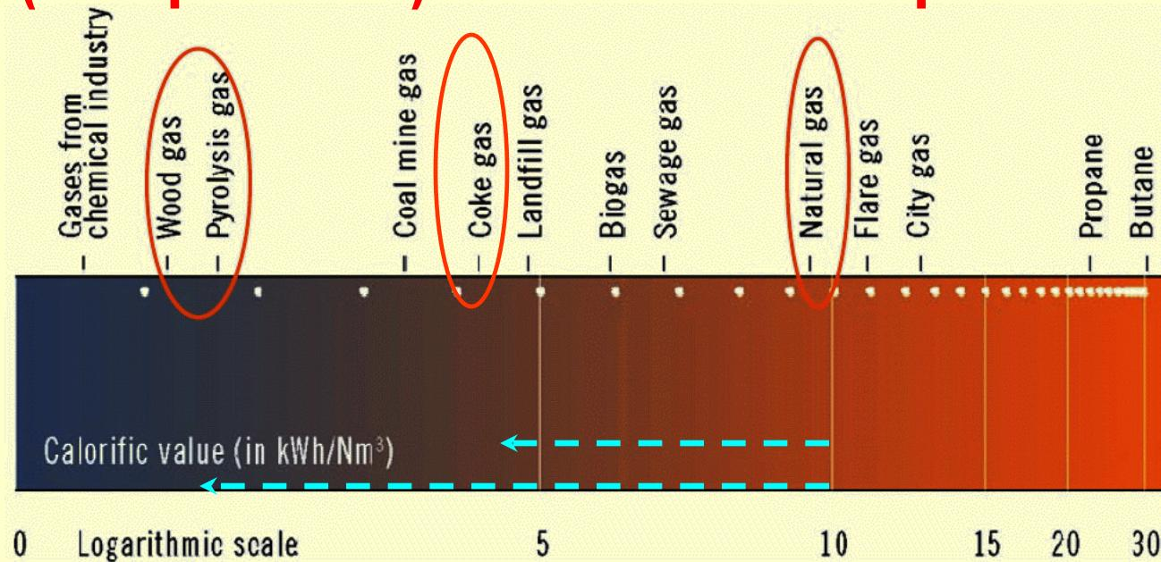
More important is a calorific value (energy content) of mixture (gas and air). Stoichiometric combustion ratio (ER =1) for different gaseous fuel (NG, LPG, SG, Wood gas) demand the different Air to Fuel Ratio (AFR).
