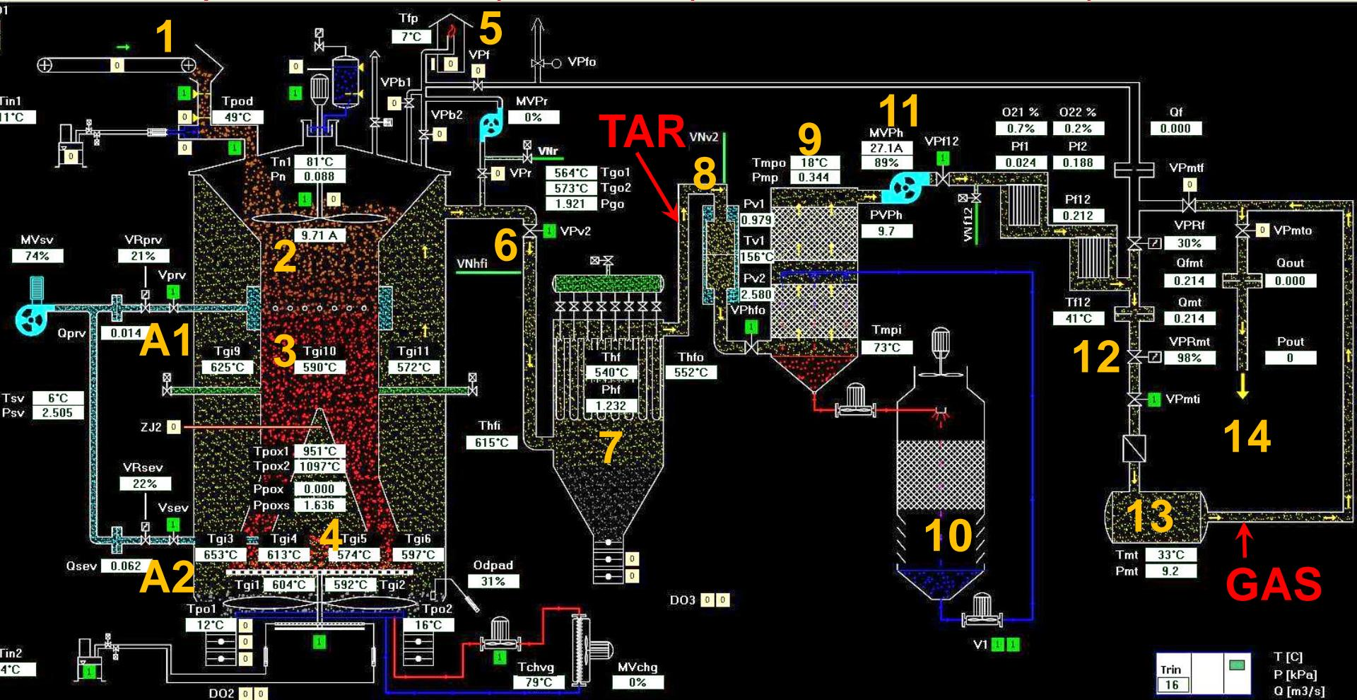
1 - entry of fuel into the GP750, 2 - allothermal pyrolysis section, 3 - autothermal pyrolysis section, 4 - POX section, 5 - combustion flare, 6 - gas output, 7 - hot filters (CERAFIL XS 3000), 8 - heat exchangers (gas/water), 9 - contact water cooling, 10 - cooling tower, 11 - gas blower, 12 - gas flow measurement , 13 - mix tank, 14 - pipe to IC motor
