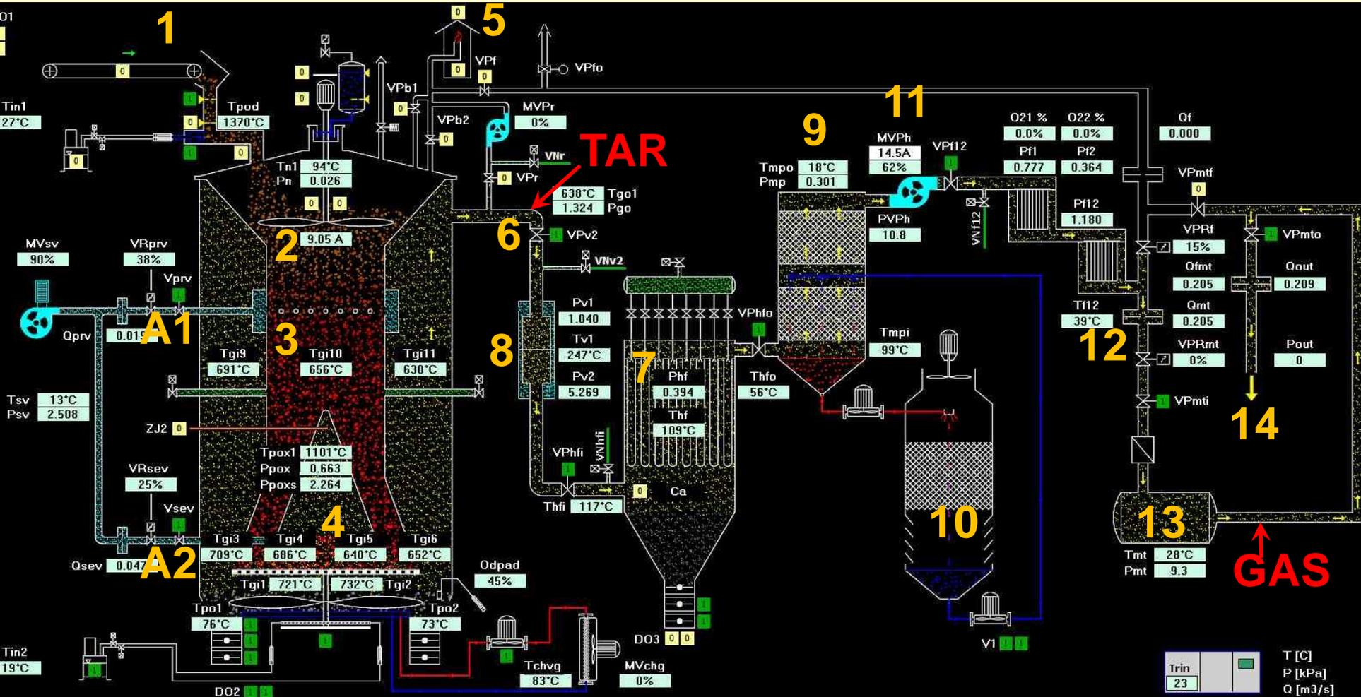
1 - entry of the fuel into the GP750, 2 - allothermal pyrolysis section, 3 - autothermal pyrolysis section, 4 - POX section, 5 - combustion flare, 6 - gas output, 7 - bag filter, 8 - heat exchangers (gas/water), 9 - contact water cooling, 10 - cooling tower, 11 - gas blower, 12 - gas flow measurement, 13 - mix tank, 14 - pipe to IC motor.
