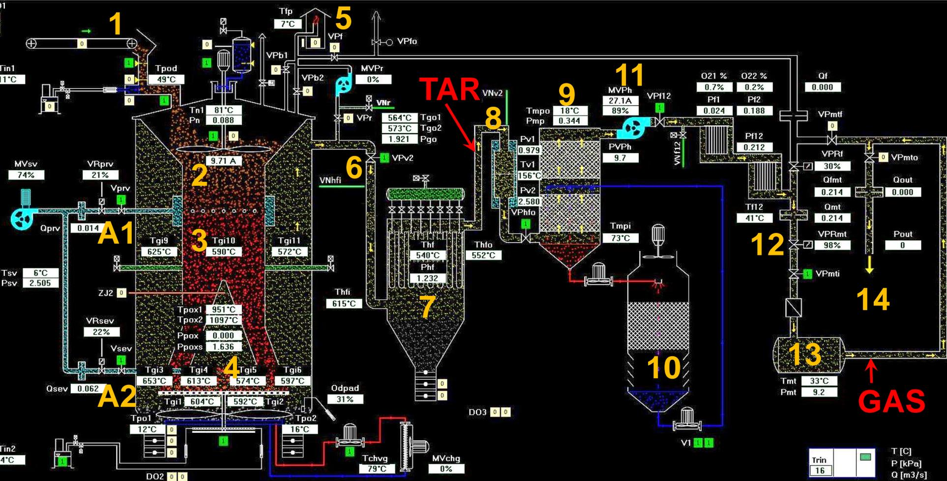
1 - entry of fuel into the GP750, 2 - allothermal pyrolysis section, 3 - autothermal pyrolysis section, 4 - POX section, 5 - combustion flare, 6 - gas output, 7 - hot filters (CERAFIL XS 3000), 8 - heat exchangers (gas/water), 9 - contact water cooling, 10 - cooling tower, 11 - gas blower, 12 - gas flow measurement, 13 - mix tank, 14 - pipe to IC motor
